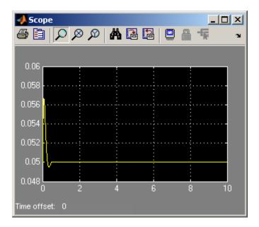
As you can see, the system is now stable and the height of the magnetic ball settles at the desired height of 0.05 m.
