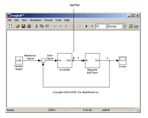
**3** Right-click the signal line after the Magnetic Ball Plant and select **Linearization Points > Output Point** from the menu.
