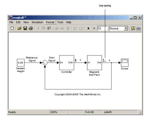
**Note** You do not need to place a loop opening in the same place as an input or output point. For example, in the following figure the highlighted blocks are included in the linearization. The loop opening is placed after the gain on the outer feedback loop, which removes the effect of this loop from the linearization. Placing a loop opening at the same place as the output point would have removed the effect of the inner loop from the linearization as well.
