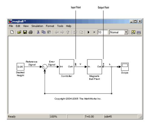
**Note** All linearization points are referenced to the output port of the block the signal line originates from. For example, placing a linearization point anywhere on the feedback loop in the figure above will result in a linearization point at the output of the Magnetic Ball Plant block.
