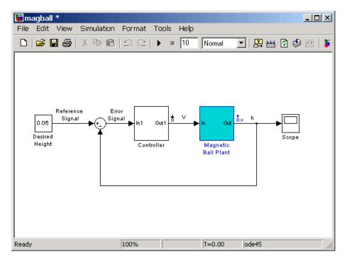
**Linearization**. The following figure shows that the Magnetic Ball Plant block, including all blocks within it, was used in the linearization.
