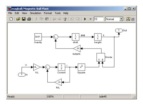
The input to the Magnetic Ball Plant system, which is also the output of the Controller subsystem, is the voltage, V. The output is the height of the ball, h. The system contains three states within the three integrators: height, dhdt, and Current.
